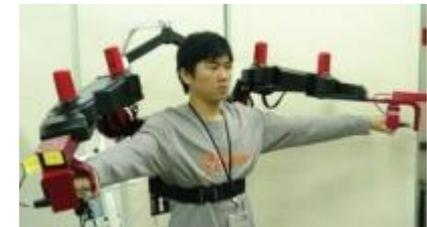
Wearable Robot for Construction Labor
