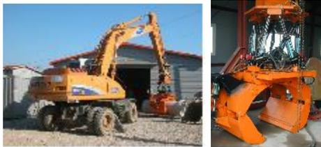
Embedding Hume Concrete Pipe Device
