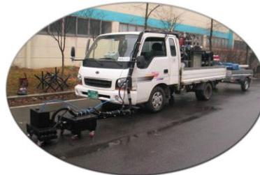
Road Stripe Removing Equipment Using Water Jet
